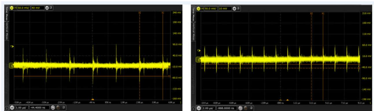
Output voltage (AC coupled) 50mV/Div
