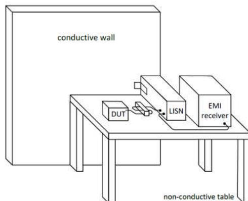
Figure 1: Test set-up for interfering voltage
