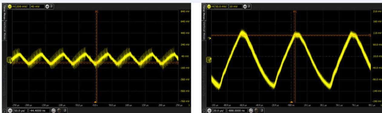
Output voltage (AC coupled) 200mV/Div
