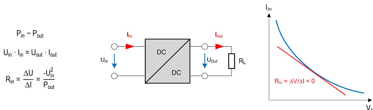
Fig. 9: Since the output remains constant even in the case of a drop in the input voltage, it is logical that the input current must rise. This results in a brief negative input resistance during this voltage transient.
